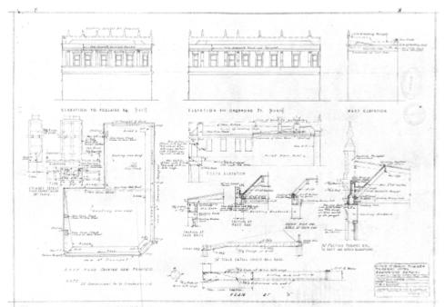
Image: B22430 Reinstatement after earthquake damage, note the lightweight parapet formed in timber framing. Plan, elevation and details. City Archives
