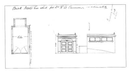
Image: 6766 Plan and elevation of Brick Motor Car Garage for Dr R G Cameron from City Archives
